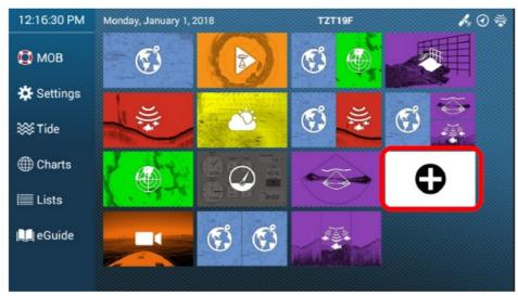
Tap on desired page layout (left hand side) then simply drag and drop applicable display to each partition. Tap on Green Check Mark to save. As a helpful tip, we recommend you set up a one of the available Function Gestures options, found in the General Menu as Full Screen to quickly switch from Quarter screen to Full screen and back from Full screen to Quarter screen.
