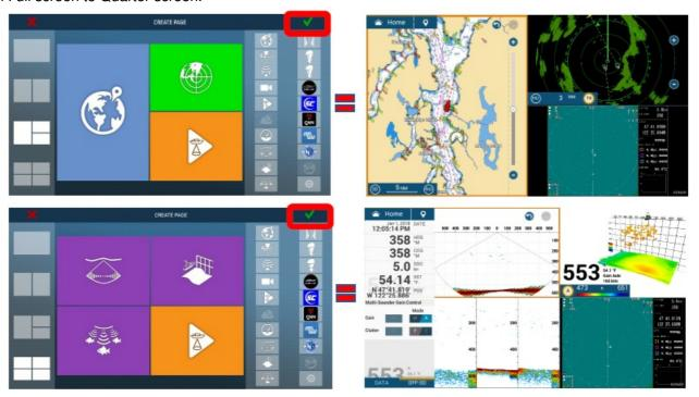
As a reminder, if you have more than one TZtouch3 MFD on the Network and wish to access the Sonar Video Stream on multiple MFDs, simply perform the setup procedure described in this document on ALL TZtouch3 MFDs.
