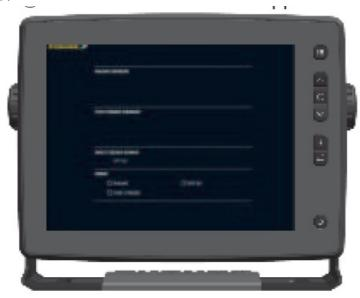
• Tap the sensor to use (RADAR SENSOR / FISH FINDER SENSOR / MULTI BEAM SONAR).
