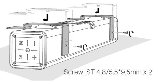
2. Place the outdoor TV face down on a flat surface with a foam board protected. Mount the outdoor soundbar with brackets to the outdoor TV using the 4 provided screws. At least two people are required for installation to avoid any damage due to the heavy weight.
