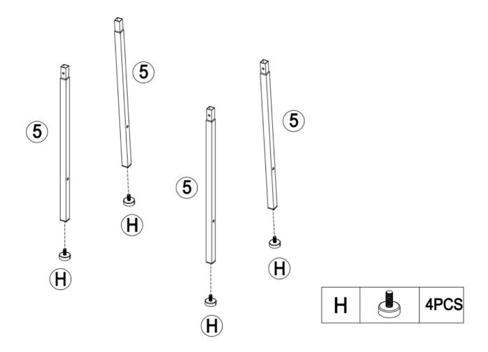
STEP 2: Fix the frames 3 and 4 to tube 5
