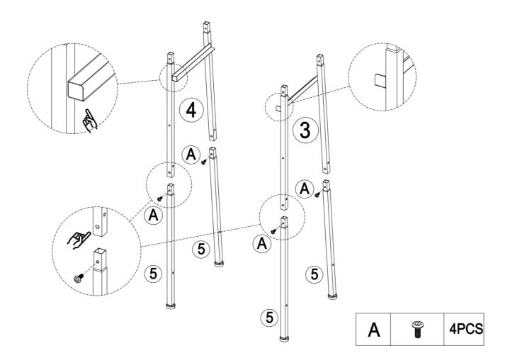
STEP 3: Fix the tube 2 to frames 3 and 4
