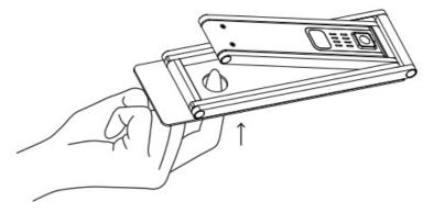
2. Lift the other side of the arm, then pull and flip the camera head in the sequence and direction indicated by arrows below.
