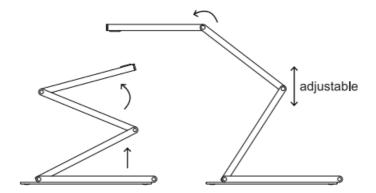
3. Adjust the camera head until it is horizontal to the shooting surface. Fully extend the arm to capture maximum shooting area of A3.
