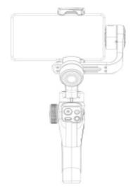
2. Vertical installation: Rotate the phone clamp 90° to the right and install it in the middle vertically.
