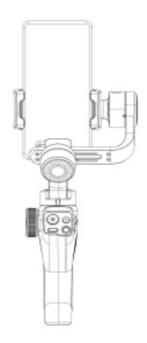
3. **Balancing adjustment:** Unlock the balance adjustment wrench on the roll axis, move the arm left or right until the phone is naturally balanced, and then tighten the balance adjustment wrench.
