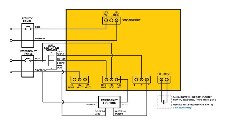
**UL924 – BYPASS WITH DALI DIMMING APPLICATION**
