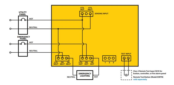
**UL1008 – SWITCH OR 2-WIRE DIMMING APPLICATION**
