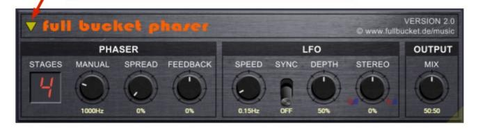
The "LFO" section controls the speed (up to 25Hz) and the depth of the low frequency oscillator modulating the Phaser frequency. The mix between original and effect is set in the "OUTPUT" section.
