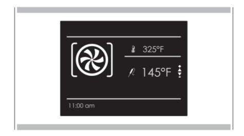
1. Set the required probe temperature by means of the arrows  $\triangle \nabla$  and confirm with the  $\bigcirc$  key.
