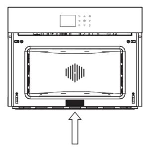
**NOTE:** Alternatively, the rating label can be placed in the upper corner of the control panel.
