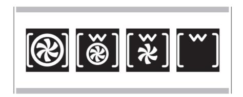
Once the oven has been turned on, the steam assist function will only become available once the internal oven temperature has exceeded 210°F (100°C). Only from that moment on will the symbol  $\clubsuit$  appear on the lower part of the display.
