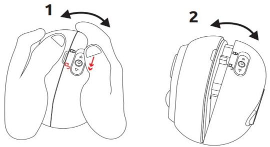
Open the housing and pull the protective tabs to activate the camera batteries.
