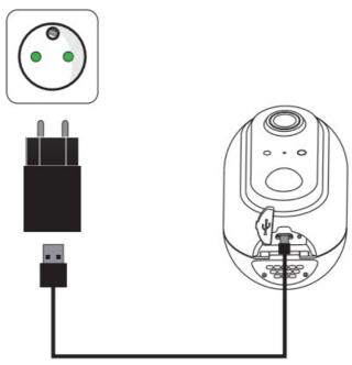
Use the supplied Micro USB cable to connect the camera to a USB power supply (not included). To obtain the correct charging time, it is recommended to use a USB charger of 1A or more. Once plugged in, the camera indicator lights red, and the batteries are fully charged when the indicator turns green.
