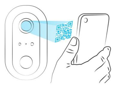
Once the code is recognised, the camera emits a confirmation beep: it is then connected to the Wi-Fi network and associated with your account.
