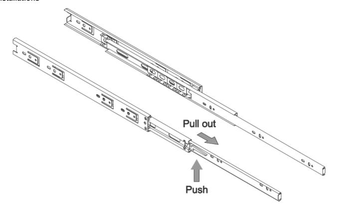
Disconnect the keyboard rail with the BLACK PLASTIC PART. It needs to be pulled down to disconnect the runners.
