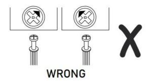
Nut should be in the centred of the cam lock when the two panels are joined. Cam lock should be inserted before nut.
