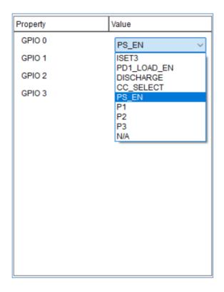
Figure 2 – GPIO Configuration options when external DC is enabled
