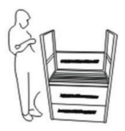
• Follow the same way to assemble batteries in the third and forth layers respectively.
