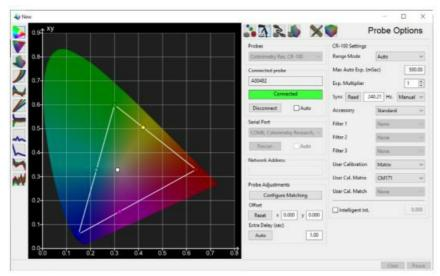
• Click on the Display Characterization icon,then select a desired profiling mode. Grey Ramp RGB Large (quick) or Cube Based
