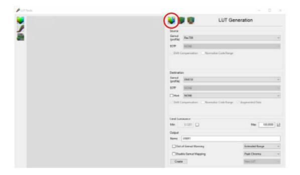
Then click create LUT. Save the LUT and then from the Manage Spaces window in ColourSpace export the LUT you just created in the [1D] FSI\_10bits (\*.lut) format. Make sure to name this 1D LUT file user1.lut then copy/paste the file to the monitor's memory.
