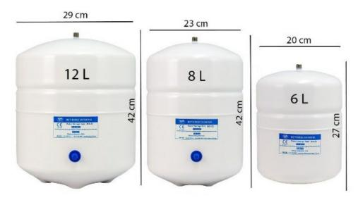
A common misunderstanding with reverse osmosis (RO) storage tanks is the difference between labelled capacity and usable water volume. For example, an 18-litre tank's total volume includes both water and air chambers, so it holds about 12 litres of water. However, due to lower RO system pressures, it might only deliver around 10 litres. As water is drawn, the flow rate decreases, so even though an 18-litre tank may contain 10 litres, only about 5 litres might be at a desirable flow rate.
