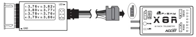
**Warning:** Install FrSky Li-Po Voltage Sensor on any appropriate surface of the airframe that stays away from water, vibration, or fuel.
