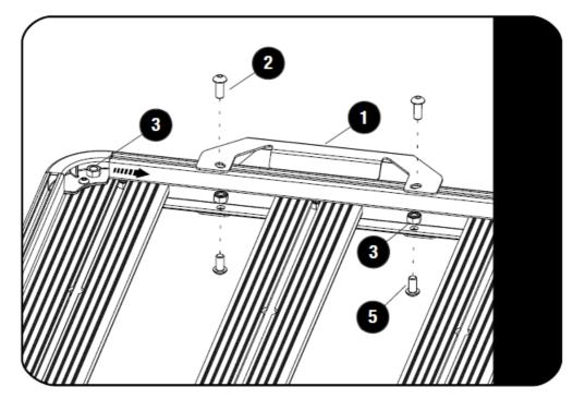
2. Secure the Handle Light Rack Bracket (Item 1) to your Roof Rack using M8x16 Button Heads, M8x30 Button Heads, M8x16x1.6 Flat Washers and M8 Nyloc Nuts (Items 2,3 & 6).
