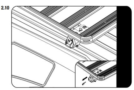
After all the feet are tightened refit the all four Feet covers.
