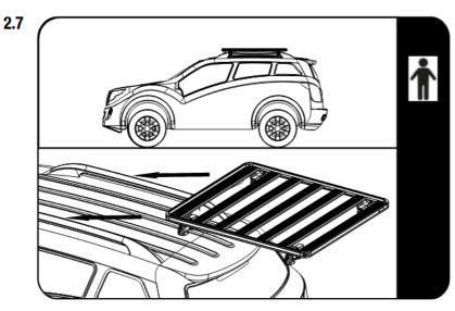
With the help of a friend, flip the rack over, right side up and place it onto the rails of the vehicle.
