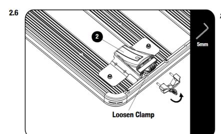
Unlock the covers on all four Feet and loosen the clamps using a 5mm Allen Key.
