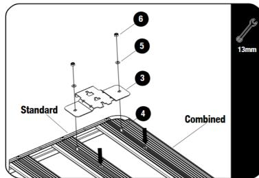
Flip the Rack so that the bottom of the Rack faces up. Insert two M8 x 16 Hex Bolts (Item 4) into the Combined slat and Standard slats machined slots as shown.
