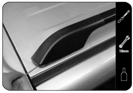
2. Apply a bead of silicone around the locating holes of the factory rubber pads before inserting 4 Rubber Inserts
