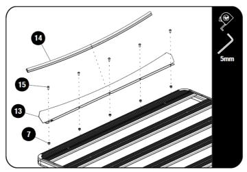
Remove one of the rack corners and then turn the rack upside down. Load the Nyloc Nuts (Item 7) into the combined slat. Loosely bolt the Wind Fairing (Item 13) to the combined slat of the rack using the M8 x 16 Button Head Bolt (Item 15) and the M8 Nyloc Nuts (Item 7). Use a tape measure to center the Wind Fairing an Fully tighten. Place the Wind Fairing Rubber (Item 14) on the Wind Fairing.
