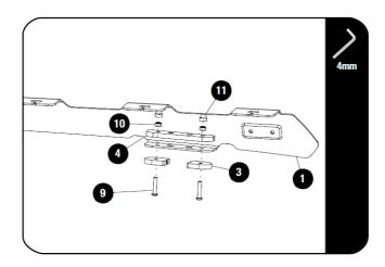
Fit the large metal spacer (Item 4) to the top of the mounting flange and the smaller plastic spacers (Item 3) to the underside of the flange as shown using M6x30 Button Head Screws (Item 9) and M6 Nylocs (Item 10).
