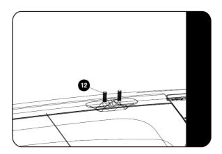
Place the M8 V Bolt (Item 12) into and around each of the four accessory ports as shown.
