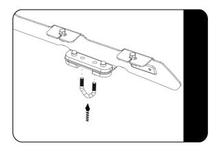
Place the Foot Rail assembled in step 2.1 over the accessory ports and insert the V bolt through the Foot Rail Base as shown. Thread the M8 Nyloc Nuts (Item 7) onto the M8 V Bolts and tighten equally alternating between the 2 nuts. Check the alignment of the plastic spacers over the accessory ports and center before fully tigtening. Do this on both the left and right hand side. Place eight M8 Nut Caps over all M8 Nuts.
