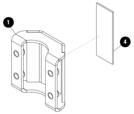
**NOTE**: Use a heat gun to heat the surface and VHB tape a little before applying. This will help to create a strong bond, especially in colder climates.
