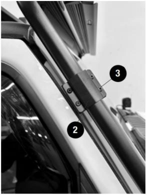
**Tightening Torque**: M6 :8- 10Nmm / 5.9 ft lb - 7.38 ft .lb
