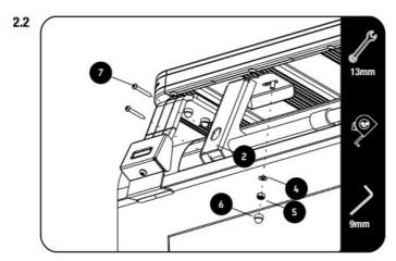
Loosely fit the Mounting Feet (Item 2 & 3) using M8 Flat Washers, M8 Nyloc Nuts and M6 x 45 Button Head Bolts (Items 4, 5 & 7) as shown.
