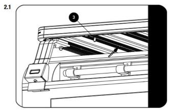
Slide M8 x 20 Hex Bolts (Item 3) into the machined slots on the 2nd, 4th, 6th & 9th slats from the rear. Referring to 2.3, remove the torx screws from the grab handle mountings on position A, B, C & D. Do this on both sides of the vehicle.
