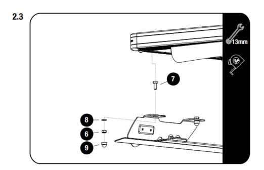
Place the Rack onto the Foot Rails (Items 1 & 2) and align the Rear Foot Rail (Item 2). Secure the Rack to the Foot Rails (Items 1 & 2) using M8 x 20 Hex Head Bolts, M8 x 12 x 1.6 Flat Washers and M8 Nyloc Nuts (Items 6, 7 & 8). Center the Rack and fully tighten all fasteners including the rearFoot Rails fasteners.
