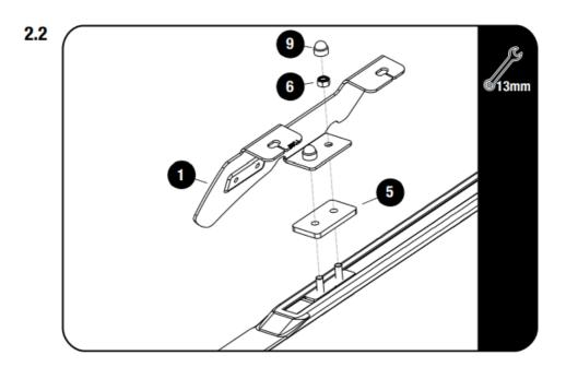
Secure the Front Foot Rail (Item 1) to the Stud Plate using 10mm Plastic Spacers and M8 Nyloc Nuts (Items 5 & 6). Push the Foot Rail all the way to the front of the channel and fully tighten.
