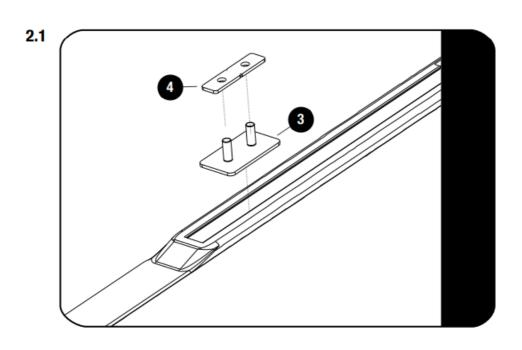
Assemble the Stud Plate and Stud Plate Spacer (Items 3 & 4) as shown. Insert the Stud Plate assemblies into the vehicle's OEM rails as shown two on the left side and two on the right side.
