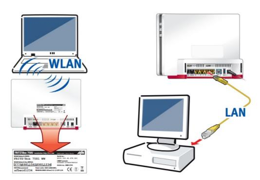
You connect computers and other network devices with the FRITZ!Box either wirelessly via wireless LAN or using a network cable. You can establish the wireless LAN connection using WPS or by entering the FRITZ!Box network key on the wireless device.
