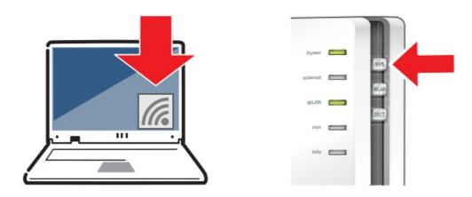
Computers with wireless LAN can be connected with the FRITZ!Box using WPS:
