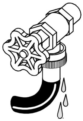
4. Determine which water faucet is the HOT water faucet and carefully connect the bottom inlet hose to the HOT water faucet, tighten by hand, then tighten another 2/3 turn with pliers. Carefully connect the top inlet hose to the COLD
