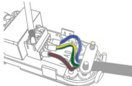
5. Attach the cable running to the appliance to the "LOAD" ports and the end which runs to the outlet into the "IN" ports)
