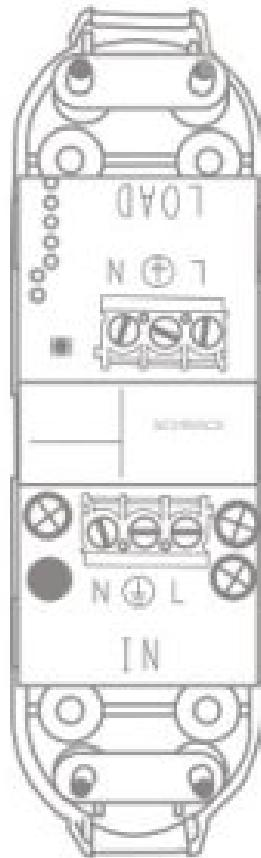
6. With the wires secured, tighten the screws of the cable clamps to secure the cable.
