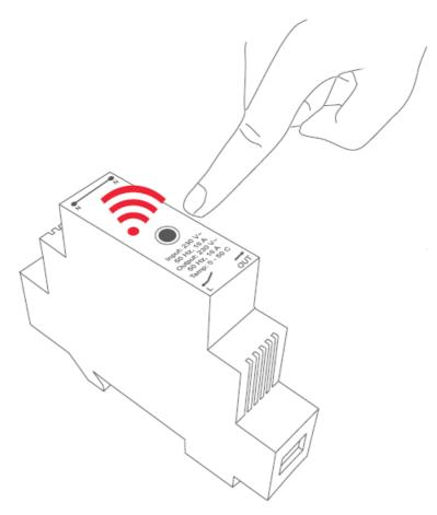
3. After releasing the button, the red LED will stay on for 2-5 seconds. During that time, the device must not be switched off or unplugged.
