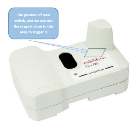
The time that magnet triggers the reed switch to connect (the duration from connect to the break) and the corresponding functions are shown in the following table:
