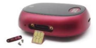
c) Replace the SIM slot cover and tighten the screws. This will ensure that the tracker is waterproof.
