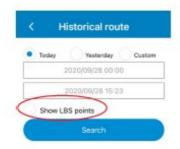
You can choose whether to filter out LBS location data (LBS location uses the nearest mobile phone tower - it is much less accurate than GPS, but can be used as a backup if the GPS location can't be found, e.g. if the person is indoors).
