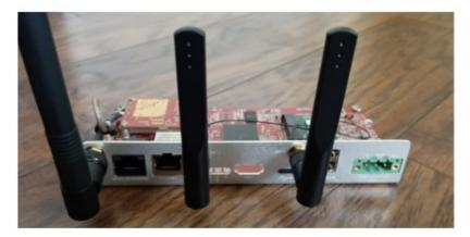
3. Finally, connect the green connector from the power supply to the front of the unit, and plug the wall adapter into a wall power source. The device will power up. On first power up, the LEDs on the device will flash in sequence several times. When boot up is complete, the LED labeled "CD" should light up and hold a steady red. The device is now ready to configure.
