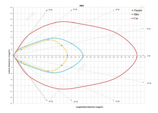
FT will provide radar mechanical 3D data along with accurate radar FOV cone. If FOV cone is interfered while installing radar on vehicle, Freetech's review and agreement shall be needed.
