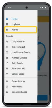
2. Touch Low Glucose Alarm and turn on alarm (alarms are off by default) Signal Loss Alarm is automatically turned on when glucose alarm is turned ON
