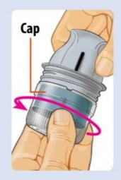
Peel lid completely off Sensor Pack. Unscrew cap from Sensor Applicator.
