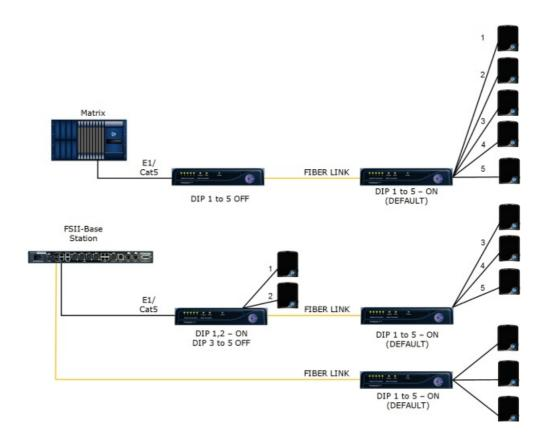
Note: Splitter daisy-chaining is not available when using E1 with an E-IPA card
