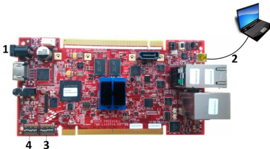
Figure 2. Switch/jumper settings and console port
