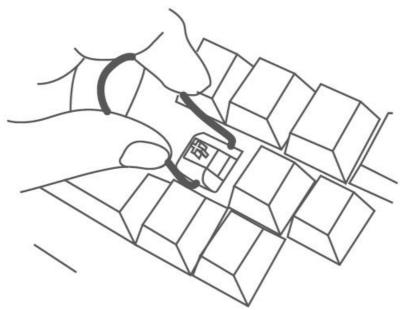
With the keycap already removed, place the switch puller over the top and bottom part of the switch and clamp it tightly while lifting it upwards.
