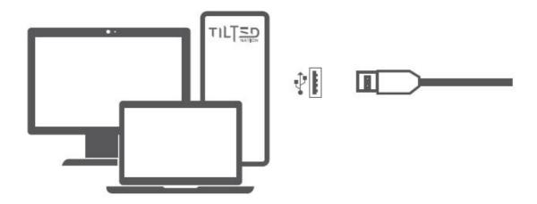
Connect the USBC end of the USB cable into the USBC slot located on top end of the keyboard and the USBA end into any available USB port on your computer or laptop. The device is Plug-N-Play and will be ready to use after the driver is automatically installed by Windows.
