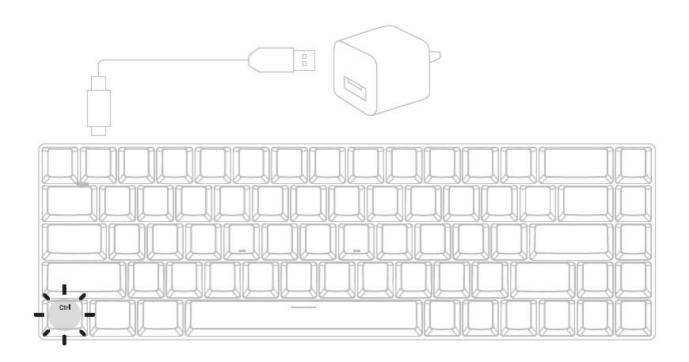
When using the keyboard wirelessly, the CTRL key located on the left side of the keyboard will start to flash indicating that the battery is low and needs to be charged. To charge the keyboard simply connect the USBC end of the charging cable into the USBC port located at the top of the keyboard and the USBA end into any USBA charger.
