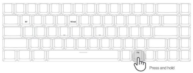
You can switch between wired and wireless mode at any time by simply holding down the FN key followed by any of the following keys:
