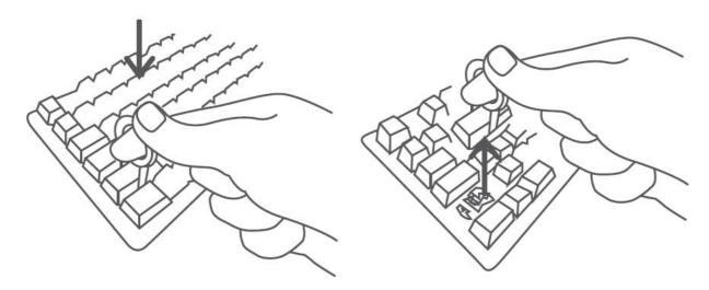
Should you need to remove the keycaps and switches on your mechanical keyboard to brush away any crumbs, dust, lint, or to simply swap out the caps/switches to add a personal touch, you'll need to use the included keycap and switch pullers.
