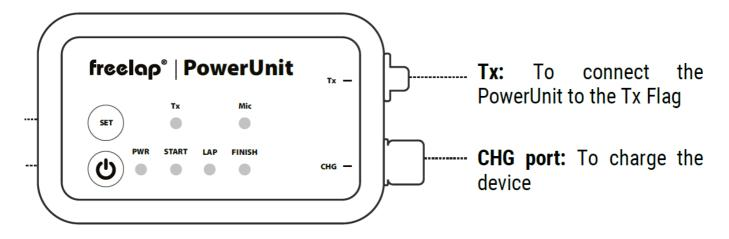
**Power button:** To turn on/off the transmitter, and to select the desired code PWR led: Indicates if the device is on (green) or if the battery is low (red) START / LAP / FINISH leds: Indicate on which code the transmitter is set.
