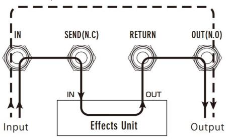
The LB-2 can be use as an output selector to choose one of two outputs. Feed signals to the IN terminal and connect from the SEND terminal to the input of an amplifier, etc. The RETURN terminal should be left unplugged. Connect from the OUT terminal to the input of another amplifier, etc. When the loop is turned on and the output 1 is selected, the output 2 is muted to preventcrosstalk or noise. Conversely, by turning off the loop and selecting the output 2, the output 1 is muted.
