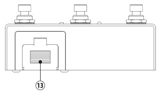
13. Holder that houses a 006P (6F22) type battery. To open the cover, slide it downward and then pull it up. When
