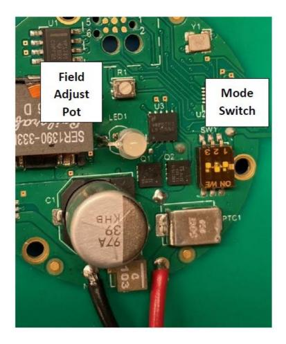
The Cab Silencer unit has three aforementioned operational modes (Cab Silencing, Aisle Identifier, or Roadway Marker) that can be selected using combination settings of the three-switch unit "SW1" on the printed circuit board. Combinations of the three switch settings allow eight different operational modes. A multi-colored LED emits flashes every 15 seconds to denote which mode is operating. The table below delineates switch combinations for the eight modes and the corresponding LED flashes.
