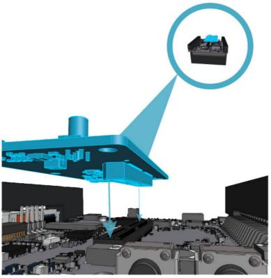
$4. \ \mbox{Connect the PixelMate}^{\mbox{\tiny TM}} \ \mbox{to the FPA.}$
