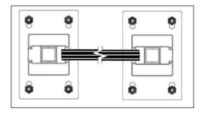
After you've placed your final fence board, insert the top cap rail (A11) into the slots of the posts. This cap rail should lock in place as shown on the right.
