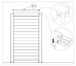
Finally, install the post caps (A5) to lock in the top cap rail and horizontal fence boards.
