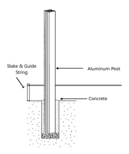
**Tip:** Wait until the concrete has completely cured before installing the rails or horizontal fence boards. Once your posts are secured, insert the bottom support rail (A10) into the slots of your posts until it rests on the board stopper.
