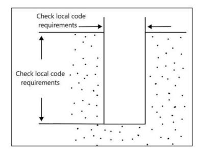
Pour 3" (72mm) of gravel into the post holes to allow drainage. Compact the gravel into the hole and ensure a level surface.
