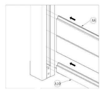
Then, slide the boards (A8) into the slots of the post. Each board should nest into the one below it. When installing the boards, it is necessary to leave a gap of 9mm | 0.3 inches between the fence board and the center rib of the posts on each side (see the figure on right).
