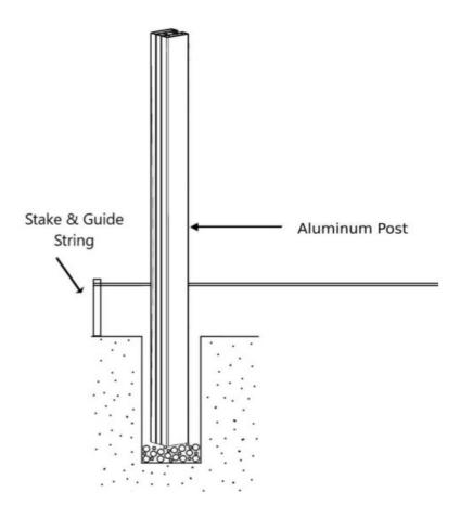
Once the post is positioned in the hole, pour concrete into the hole. Dome the concrete around the post to prevent water pooling over time.
