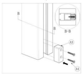
Then using the marks, pre-drill holes into the post and secure the board stopper with the screws provided (A4). The board stopper must be above ground. Take care to precisely measure to portion of post that will be underground and install board stopper appropriately. The position of the board stopper must be consistent across all posts and will determine the amount of space under your fence panels.
