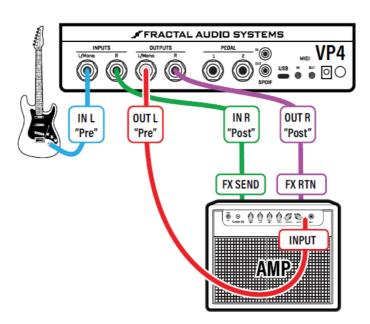
Use standard guitar patch cables for each connection. Always connect all four cables when using 4CM or it won't work.
