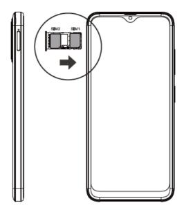
Put 1 or 2 nano-SIM cards onto the SIM tray with the gold contacts facing down and the edges match the positions on the SIM tray.
