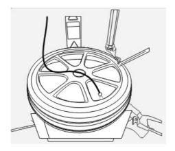
Dismantle the valve core with valve core removal tool. Then inflate the tire to the nominal value according to the tire data plate the vehicle. Install the valve core and screw the valve cap
