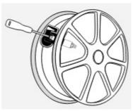
3. Use the tire valve stem puller to pull the sensor to the proper position.
