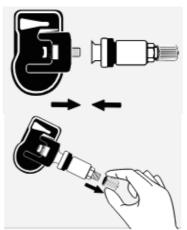
2. Remove the cap, screw nut, and grommet from the stem one by one.
