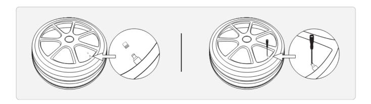
Remove the valve cover and valve core to deflate the tyre.
