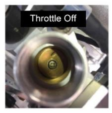
2. The EFI system does not require an additional special flameout switch. When the throttle valve is fully closed, the engine will stop and turn off, and the power to the oil pump will be cut off at the same time.
