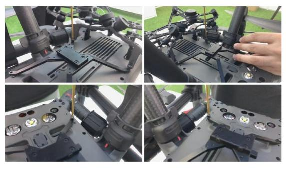
Install the five-hook release and drop device into the quick release plate, push it in after alignment, hear a click to indicate locking, and then shake the drop device to confirm if the installation is secure.
