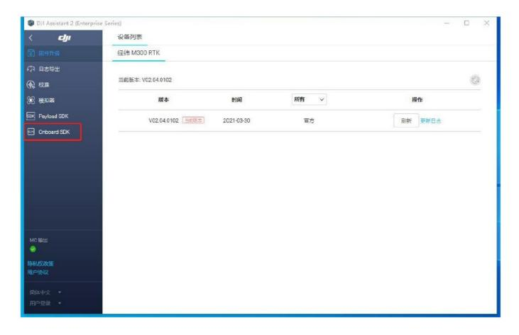
Click Onbiar SDK again, check the API checkbox, and change the baud rate to 230400. Then close the parameter configuration software, complete the drone parameter settings, unplug the type-c cable and power off thedrone.
