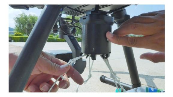
When the camera is vertical to the ground, click the SW1 icon on the left side of the APP to start the drop. When the click button is blue, it is the drop state, and when it is gray, it is the lock state. Open the 5 drop hook in sequence by clicking multiple times to drop items. After returning to the take-off point, you can load a new item using the physical button, or use the SW1 icon in the APP interface to control the opening of the drop hook.
