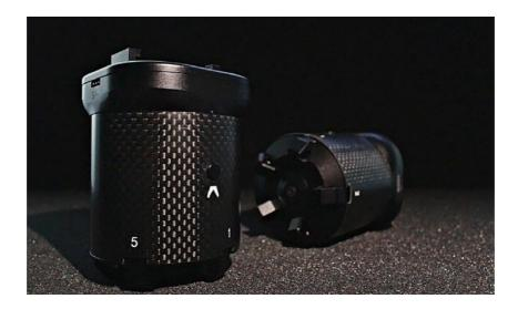
The nain body of the device is made of carbon fiber and aerospace aluminum materials, adopting CNC process, anodized and laser engraved surface treatment, waterproof and rust-proof. The device is connected with UAV OSDK through TYPE-C. There is a manual button on the device to control the hook on and off, can quickly complete payload mounting.
