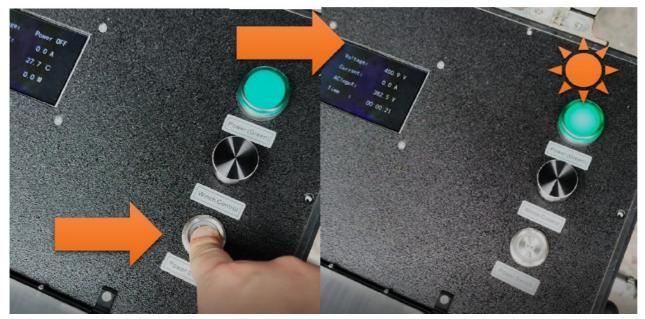
**Attention.** Please watch the green light on during the drone is hovering. If the green light is off, it means the tether power is off. The drone is powered by the battery now.
