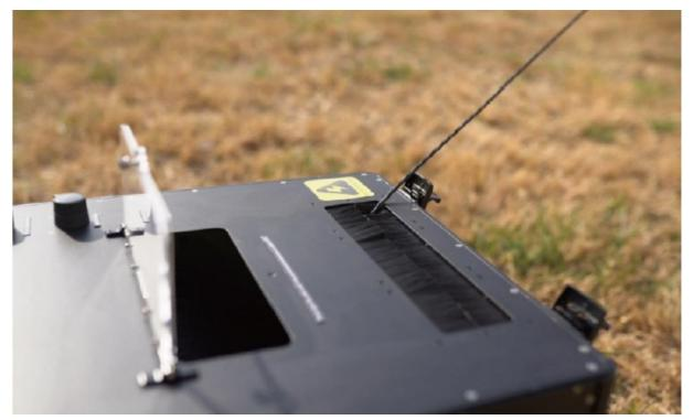
**Attention.** For inside cooling, the observation window must be open, and release the tether cable more than 80% of the total length.
