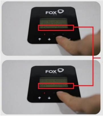
Select "factory reset" Select "set" to rest the inverter By this step, all work has been completed. Please remove the power supply and pack the inverter! Thank you very much!
